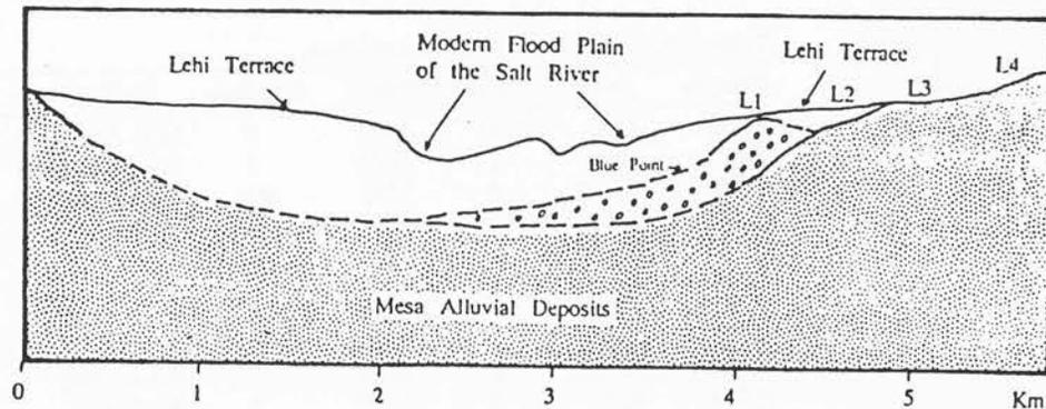
Figure 2. Geological cross section of the Salt River in the vicinity of the Tempe Outer Loop Corridor. Hohokam canals were dug on the Lehi Terrace surface (after Katzer, 1989).
